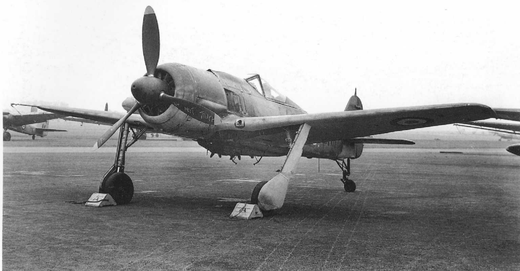
176: Shown in the display of captured German aircraft held at Farnborough in October 1945, this Fw 190F-8/R15, Werk Nummer unknown, was captured at the German marine testing station at Travemünde. Given its anonymous finish, it is possible that it was used by III/KG 200. The lengthened tail wheel which gave clearance for an under-fuselage torpedo or bomb is clearly visible. Presumably it was also fitted with the strengthened undercarriage. Given the Air Ministry number AM 111, its ultimate fate is unknown
