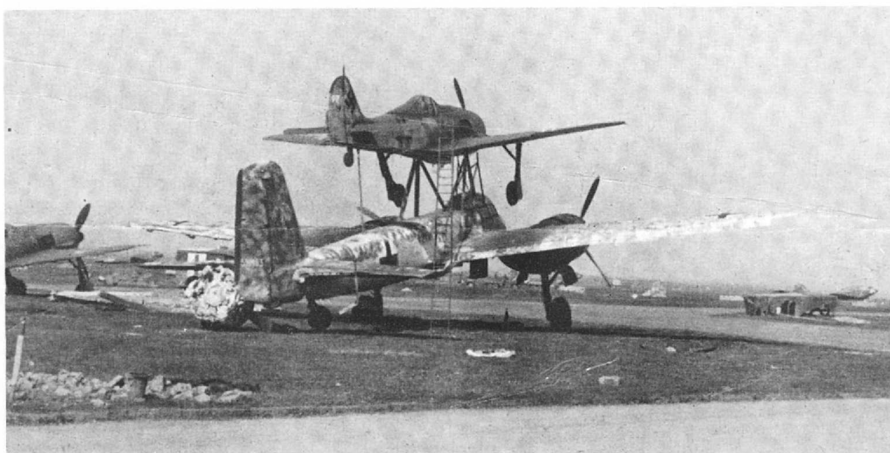
118: A Mistel 2 combination of Ju 88G-1 W.Nr. 590153 and Fw 190A-8 '97' at Merseburg at the end of the war. Just getting into the Fw 190 was an effort using the rather precarious ladder seen propped against the starboard wing. The Ju 88 was apparently once in service with NJG 5, whose 'C9' code was still faintly visible on the fuselage
