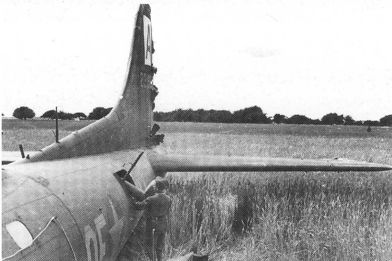
71: This view of the tail unit of 42-3190 clearly shows the extensive damage to the control surfaces. While this obviously caused severe problems for the pilot, the damage was relatively easy to repair and the aircraft was soon in service with KG 200
