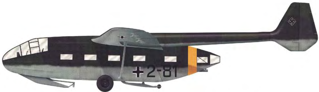
11: A Gotha Go 242, in typical glider finish, which still retains yellow Eastern Front tactical markings. It is believed that this aircraft took part in the Vercors operation. Source: Photo
